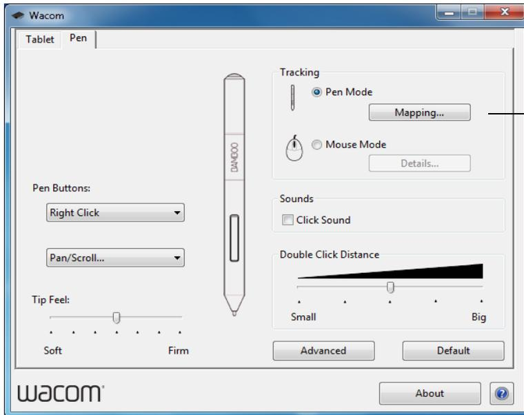
TRACKING options control how the screen cursor moves:
