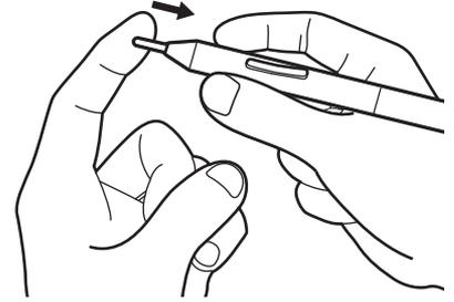
2. Slide the end of the new nib straight into the barrel of the pen. Firmly push the nib until it stops.
